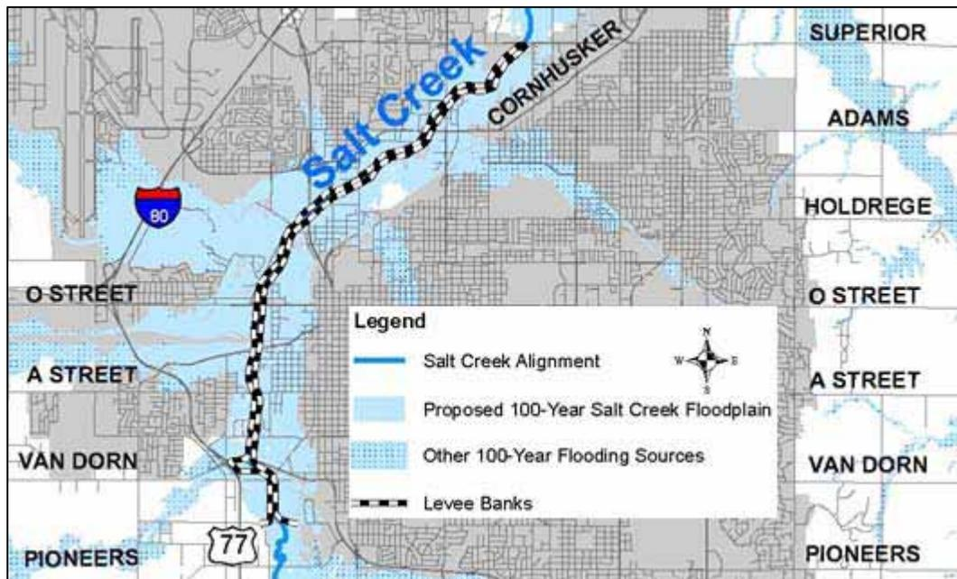
Figure 1 – Levee System in Lincoln, Nebraska
