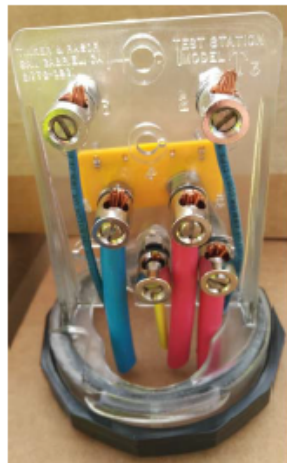
Side 1: Wire and Cable Binding Post Connections
