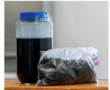
Comparison of biosolids: liquid form in a clear jar versus dry, soil-like biosolids in a plastic bag.
