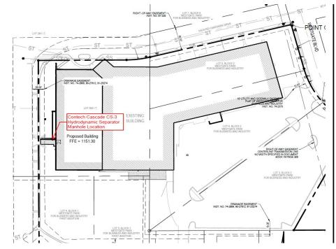
\*\* When choosing a PCBMP, keep in mind the accessibility for maintenance. If a vac truck can't access a separator, how is it going to be cleaned?
