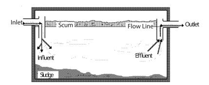
Many traps will have a layer of *scum* floating on the water surface. This layer should remain above the *flow line* (the level at which water may flow out of the tank) so that it is not released with the effluent. You should periodically check the level of scum in the tank to ensure that too much does not build up. Occasionally, this scum will include a film of oil. You should remove this oil occasionally. This oil should be reported as a special waste and disposed of properly.
