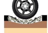
The weight of vehicles breaks the pavement which then collapses to form a pothole.
